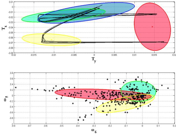
Figure 4: Resulting 4-states HMM trained with demonstrations starting at every position inside the box. *Top*: Input space composed of the most relevant inputs  $\{T_x, T_y\}$ . *Bottom*: Output space composed of robot joint velocities playing the most important role for the given task. The small, hard-to-see blue state is centred in  $(0,0)$ .
