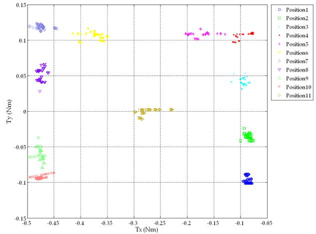
Figure 3: Torques map representing clusters for each initial position of the ball inside the container. Displaying samples of the most relevant variables to the current task  $T_x$  vs.  $T_y$ , shows that they do describe where the ball is in the box.
