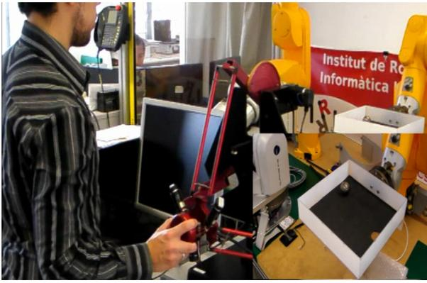
Figure 2: Experimental setup: the teacher holds the end-effector of the haptic device and teleoperates the robotic arm for teaching the task, while feeling forces/torques sensed at the robotic wrist. *Bottom right*: the box held by the robot.
