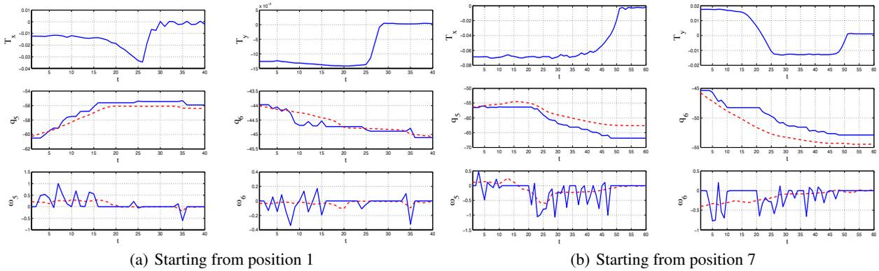
Figure 5: *Top*: Input torques  $\{T_x, T_y\}$  during demonstrations. *Middle*: Robot joint trajectories corresponding to the teacher’s demonstration (*blue solid line*) and the robot’s execution using the HMM/GMRa approach (*red dashed line*). *Bottom*: Robot joint velocity profiles obtained from teacher and robot executions, the latter computed through GMRa.
